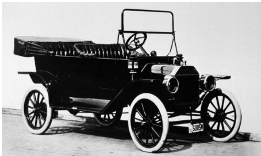
The 1914 Model T touring car - the very first version build on Henry Ford's assembly line. It was powered by a 4 cylinder 20 HP gas engine with a two speed transmission. $550 each.
